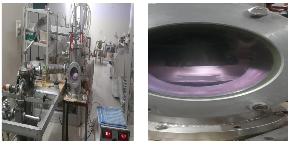
Fig. 1. A. plasma discharge treatment chamber (left) B. mustard seeds undergoing in a plasma reactor (right)
