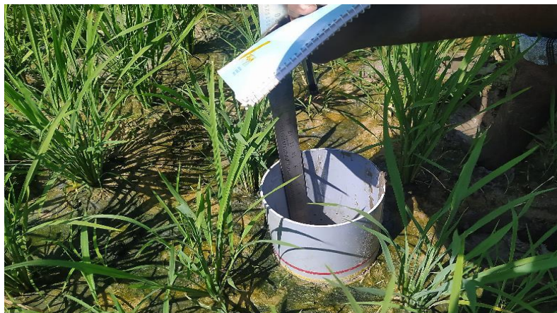
Fig. 1. Field water tube installed in AWD plots to monitor water depth
