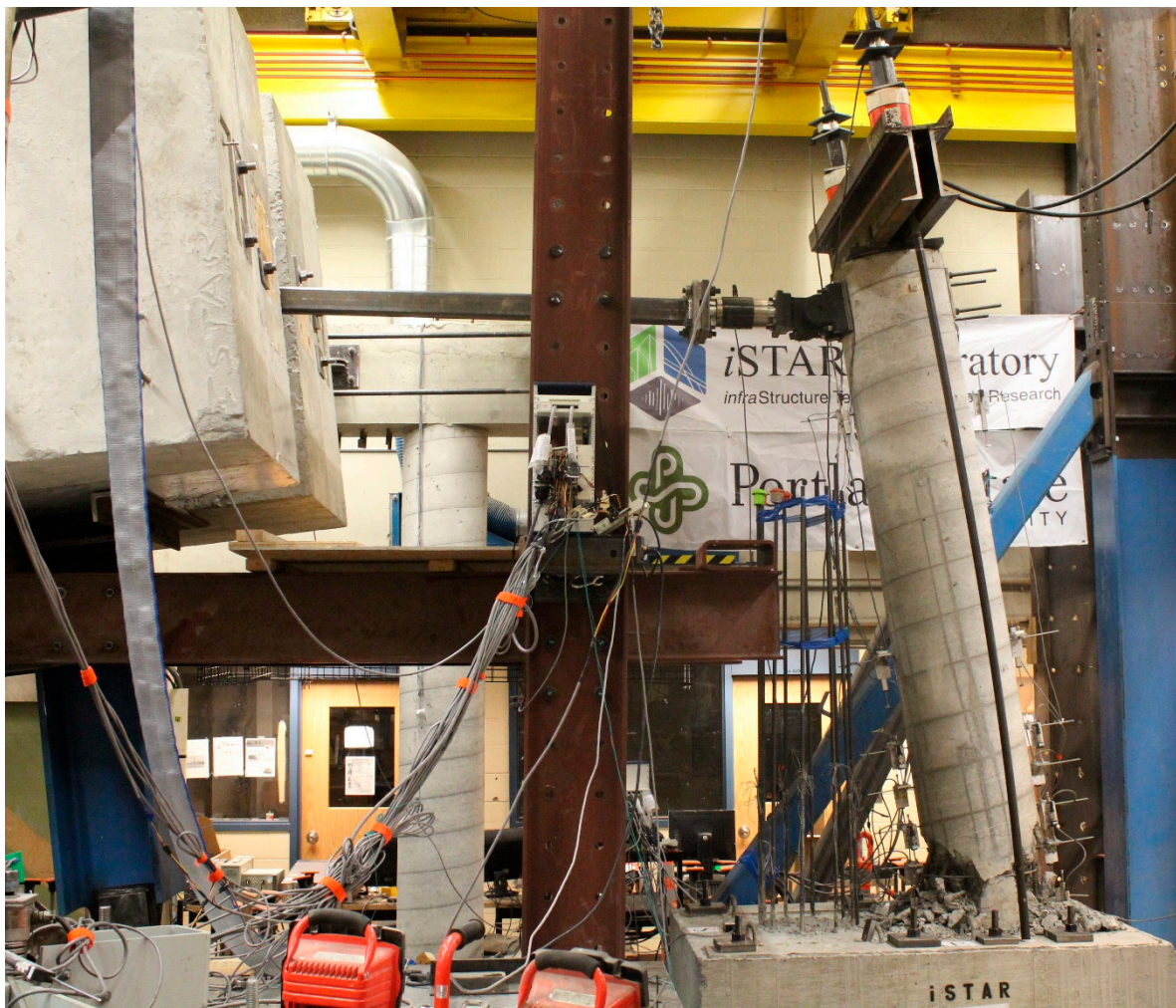
Figure 7. IMS reaching the maximum displacement limit under specimen collapse.
