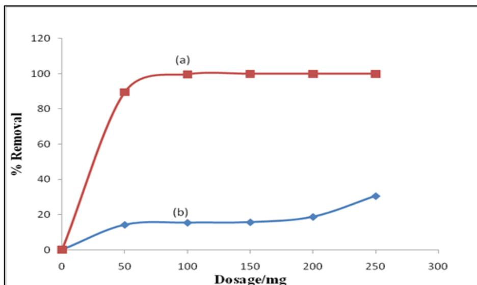
Fig. 8. Effect of adsorbent dosage on MO removal (a) using Fe<sub>2</sub>O<sub>3</sub>-BC and (b) using BC
