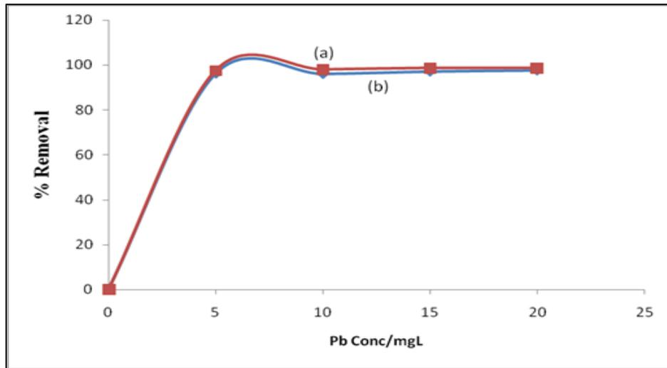
Fig. 7. Effect of adsorbate concentration on Pb<sup>2+</sup> removal (a) using Fe<sub>2</sub>O<sub>3</sub>-BC and (b) using BC
