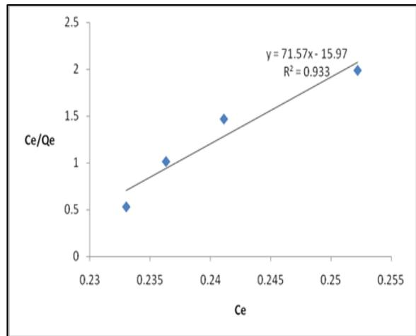
Fig. 11. Langmuir Plot for Pb<sup>2+</sup> results
