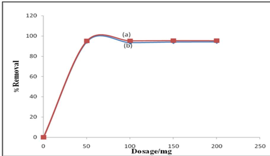
Fig. 9. Effect of Adsorbent dosage on Pb<sup>2+</sup> removal (a) using Fe<sub>2</sub>O<sub>3</sub>-BC and (b) using BC
