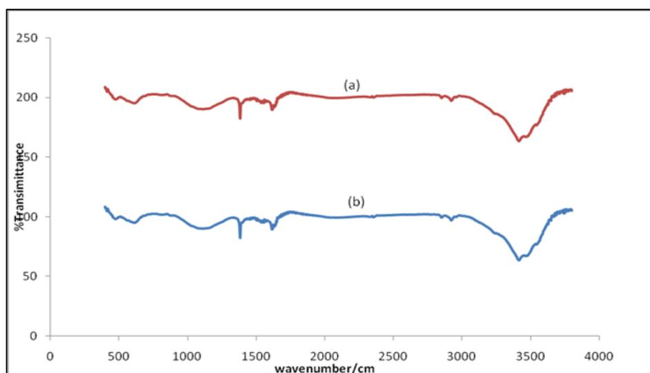
Fig. 1.  $\text{Fe}_2\text{O}_3\text{-BC}$  FTIR spectra (a) after adsorption and (b) before adsorption
