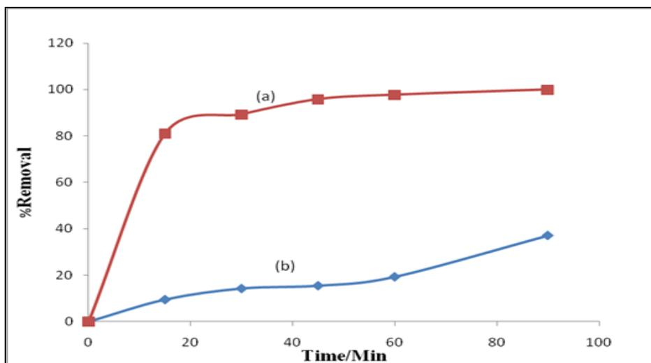
Fig. 4. Effect of contact time on MO removal, (a) using Fe<sub>2</sub>O<sub>3</sub>-BC and (b) using BC
