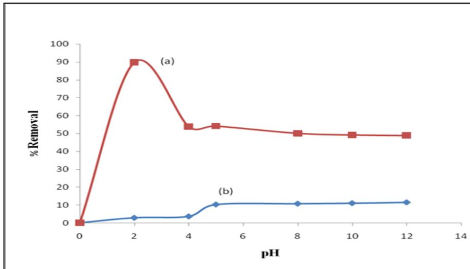
Fig. 3. Effect of pH on MO removal, (a) using Fe<sub>2</sub>O<sub>3</sub>-BC and (b) using BC
