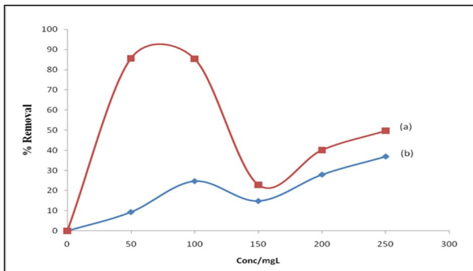
Fig. 6. Effect of adsorbate concentration on MO removal (a) using Fe<sub>2</sub>O<sub>3</sub>-BC and (b) using BC
