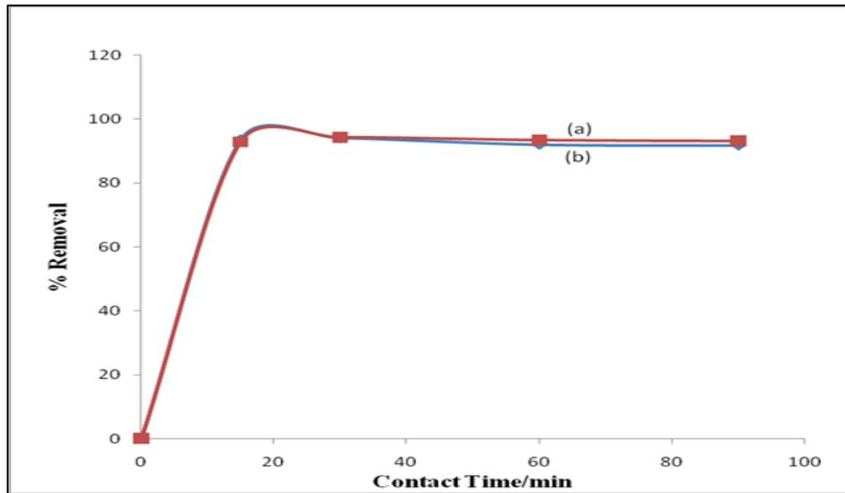
Fig. 5. Effect of contact time on Pb<sup>2+</sup> removal (a) using Fe<sub>2</sub>O<sub>3</sub>-BC and (b) using BC
